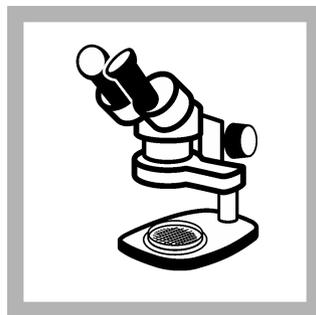
11. Remove the petri dish from the incubator. Use a 10 to 15x microscope to count the number of bacteria colonies on the membrane filter. Refer to [Interpret and report the coliform results](#) on page 5.
